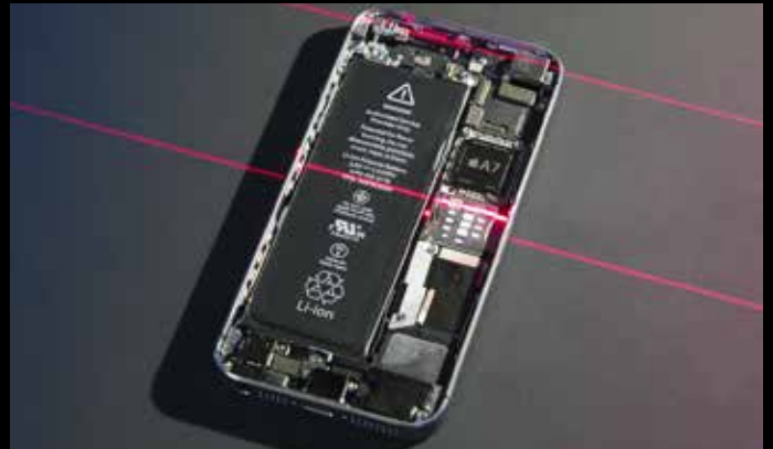
Contactless high-precision reconstruction of the DUT surface using LASER-triangulation based advanced computer vision techniques.
